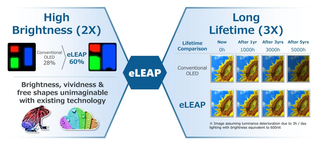
Using eLEAP's lithography with maskless deposition process instead of conventional OLED's FMM (fine metal masks) will reduce OLED production costs by c. 30%
